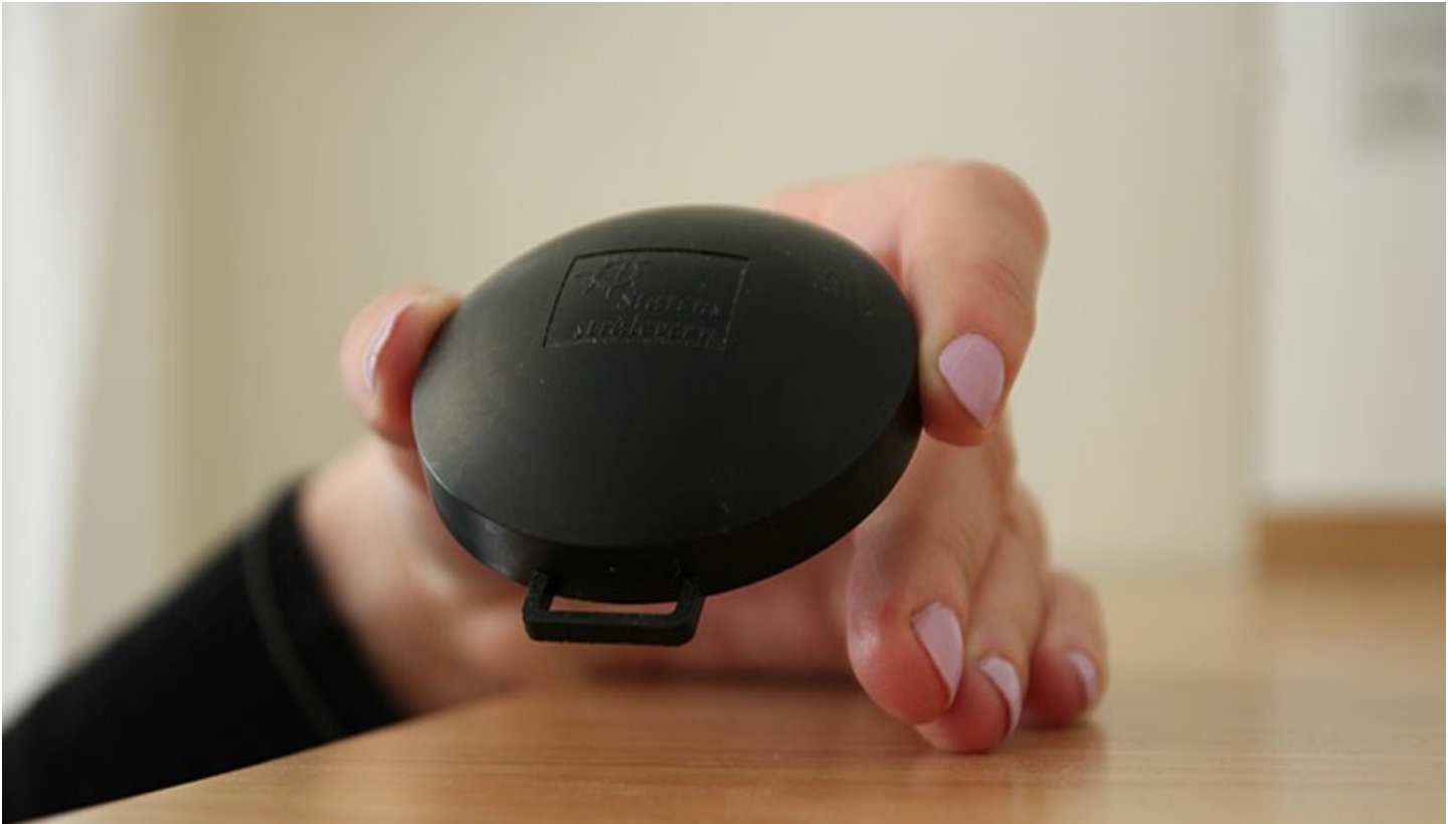
Radon in the home accounts for about half of all radiation exposure for the average Norwegian. The authorities recommend measuring radon levels in the home, using a track-etch detector as shown here or an electronic device. Photo: Norwegian Radiation Protection Authority
