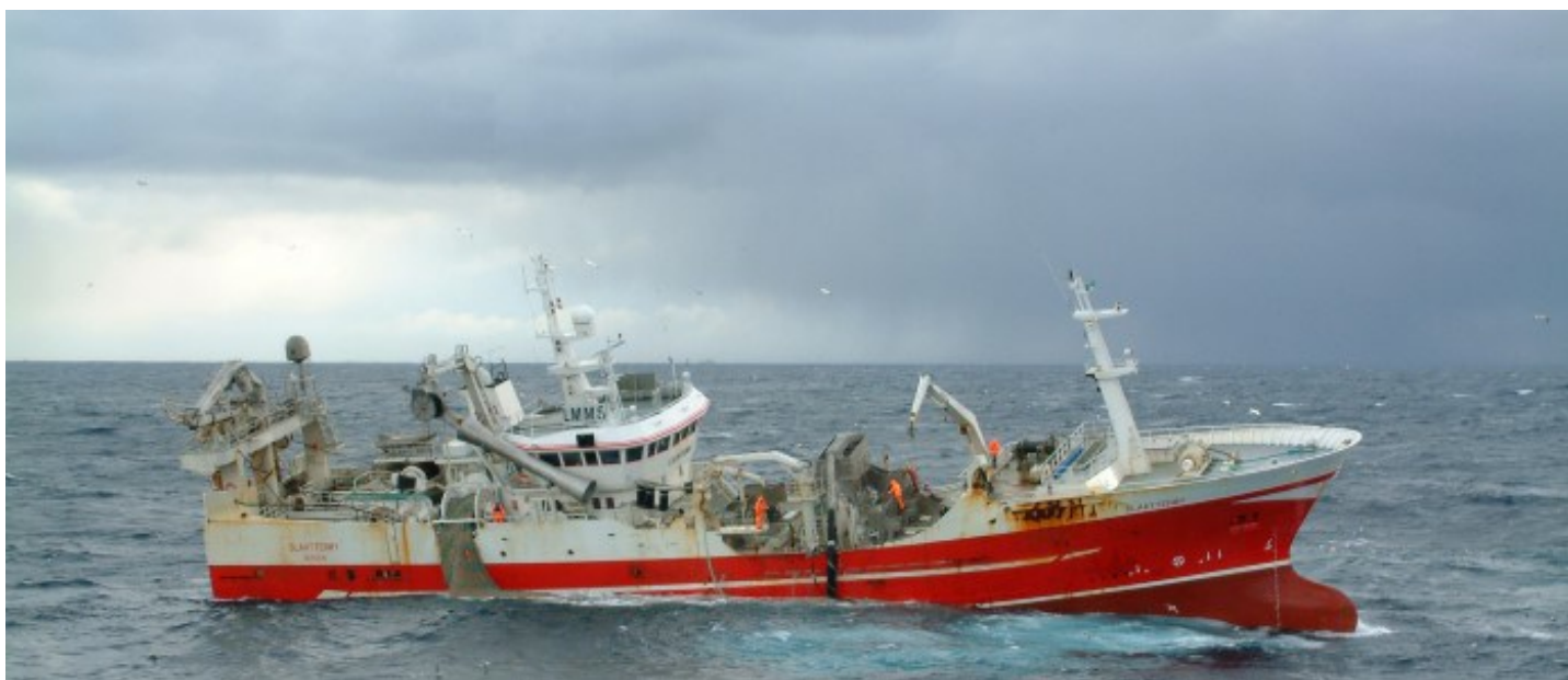
The purse seiner/trawler Slaatørø fishing for blue whiting west of Ireland. Photo: scanfishphoto.com
